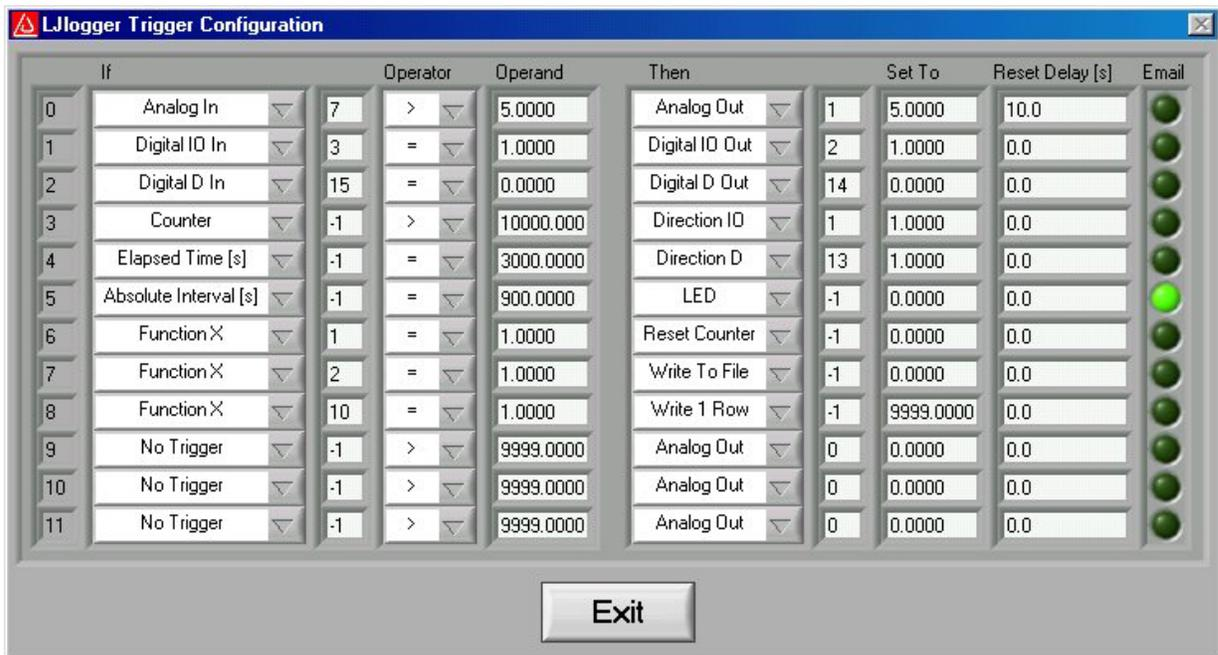
Figure 3-9. LJlogger Trigger Configuration
