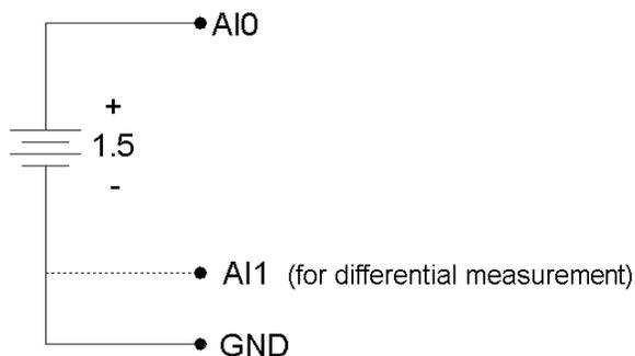
**Figure 2-2. Single-ended measurement.**
