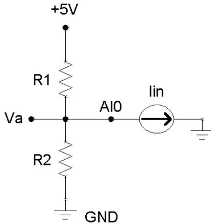
**Figure 2-4. Single-ended measurement with voltage divider circuit.**
