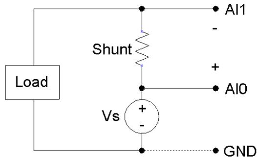
**Figure 2-3. Differential measurement.**
