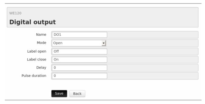
For entering the configuration page of a digital output, click on the relevant line of the table.
