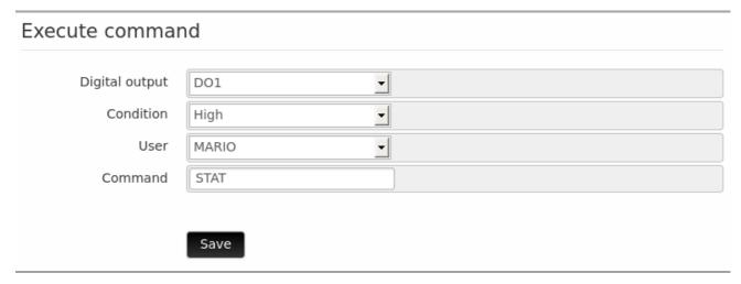
From this area it is possible to allow the WE120 to execute a command when a digital input reaches a defined value.
