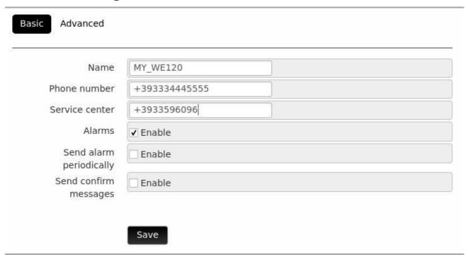
This area allows to set the general basic parameters of the WE120:
