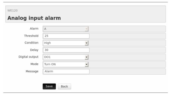
From this configuration page it is possible to program an alarm on an analogue input, setting the following parameters:
