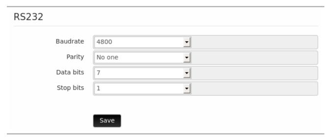
In this section the parameters of the RS232 serial port are configured:
