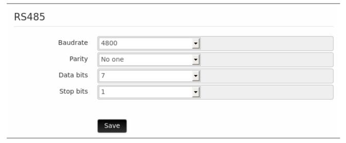
In this section the parameters of the RS485 serial port are configured:
