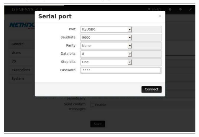
The parameters of the port used for the communication between the WE120 and the PC must be entered.
