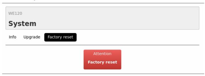
Using this button it is possible to clean all the device configuration. All the previous configuration will be lost except the serial port parameters. If a firmware upgrade was executed before the factory reset, that firmware will remain.
