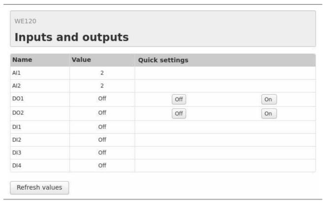
In the table is given the name and the value and, in case of the digital outputs, also a tab for activating or deactivating the output.
