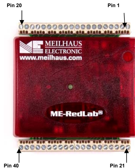
Figure 4. RedLab 1608FS screw terminal pin numbers
