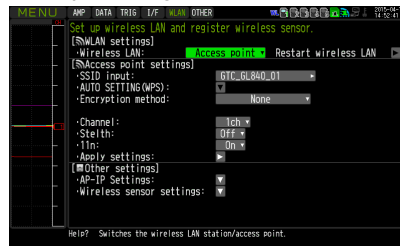
Access point settings
