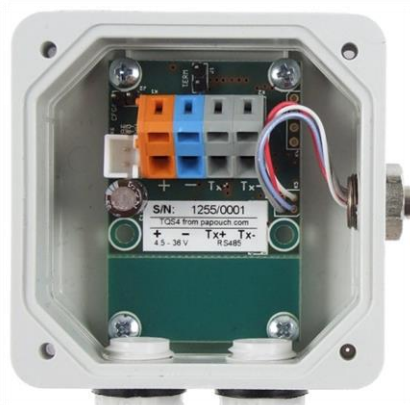
fig. 2 – Terminal block inside the box
