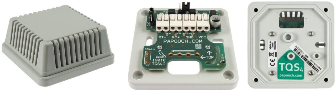
fig. 10 - TQS4 I: boxed; PCB inside; mount holes placement with cable feed-through holes
